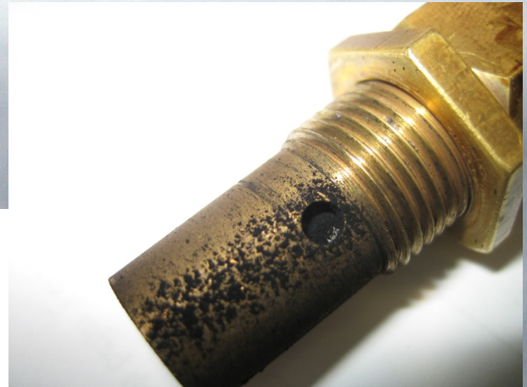
SDSS v.13 after measurements with high soot concentration
