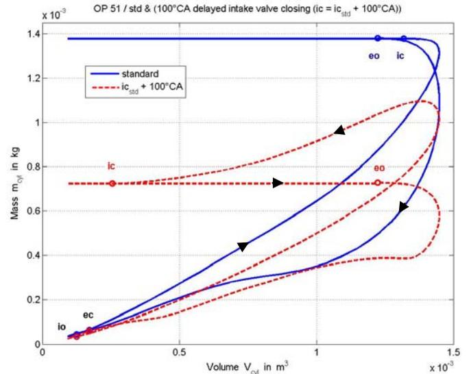
Figure 5 (gas mixture) Mass-Volume diagram (SV & 1V)
