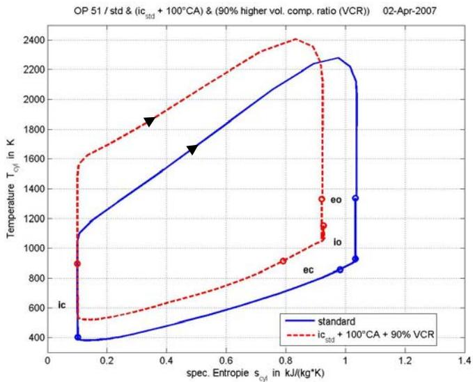
**Figure 8** Temperature–(specific) Entropy diagram (SV & 2V)
