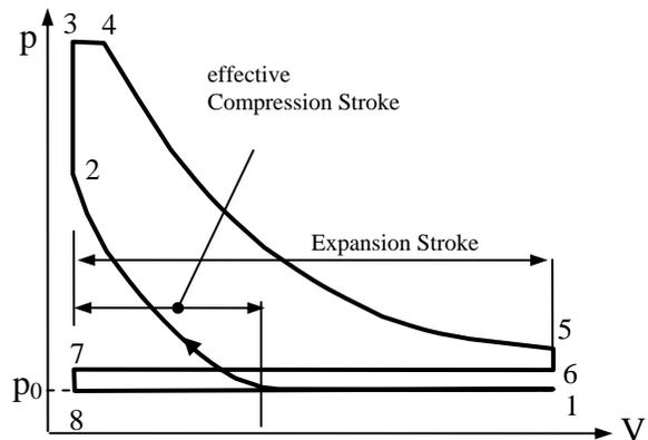
**Figure 2** Schematic Pressure-Volume diagram of a **modified** (i.e. four stroke) Atkinson cycle
