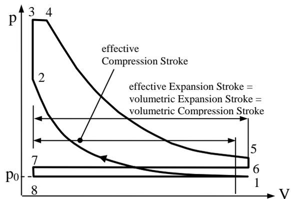
**Figure 1** Schematic Pressure-Volume diagram of a classical four stroke cycle of conventional ICE
