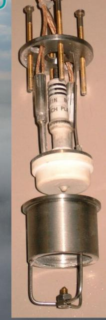
Soot sensor prototype built form many parts
