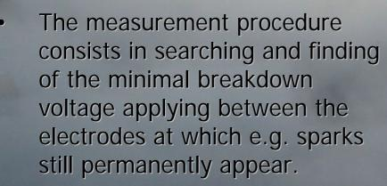
• This voltage level is considered as measure of the soot and particle concentration.
