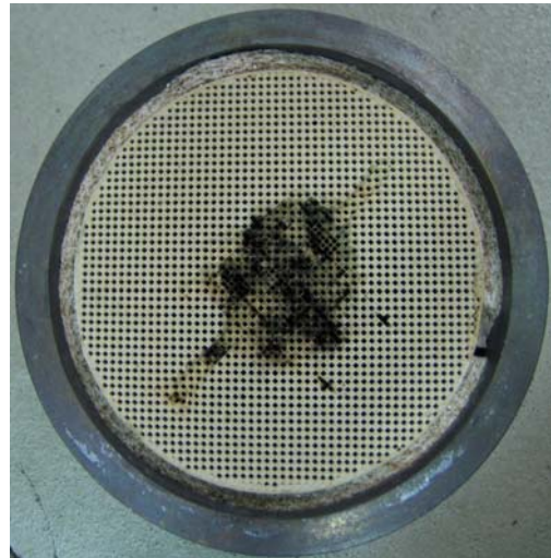
Figure 13: Damaged DPF after use in exhaust gas system. The filter was mechanically manipulated to allow direct passage for the exhaust gases and therefore for the soot particles through the middle of the filter.
