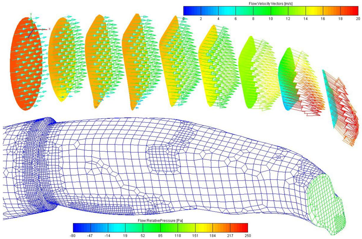
**Fig. 3** Intake channel computing mesh with relative pressure and flow velocity vectors distributions in some sections by 0.03 kg/s forward mass airflow
