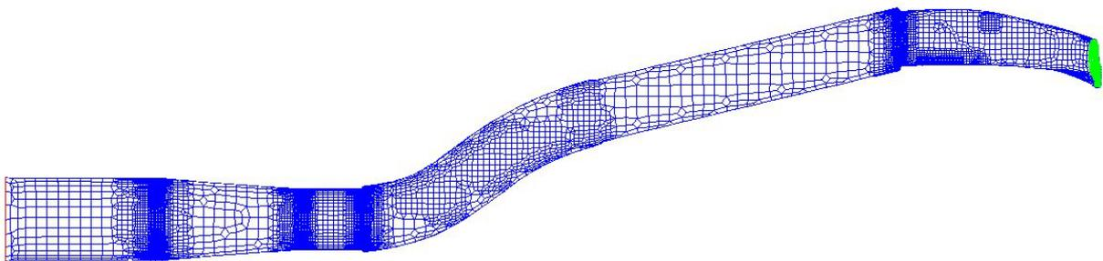
Fig. 2 Computing mesh of the all intake pipe
