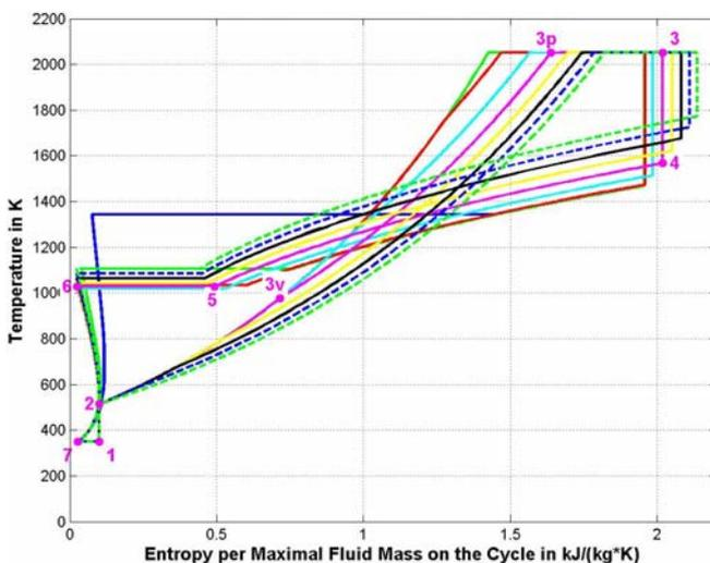
**Figure 14.** Temperature-Entropy per maximal Fluid Mass Diagrams ( $T,s^*$ ) for the Crank Mechanism in Position 1, at many Loads, AFR = 1
