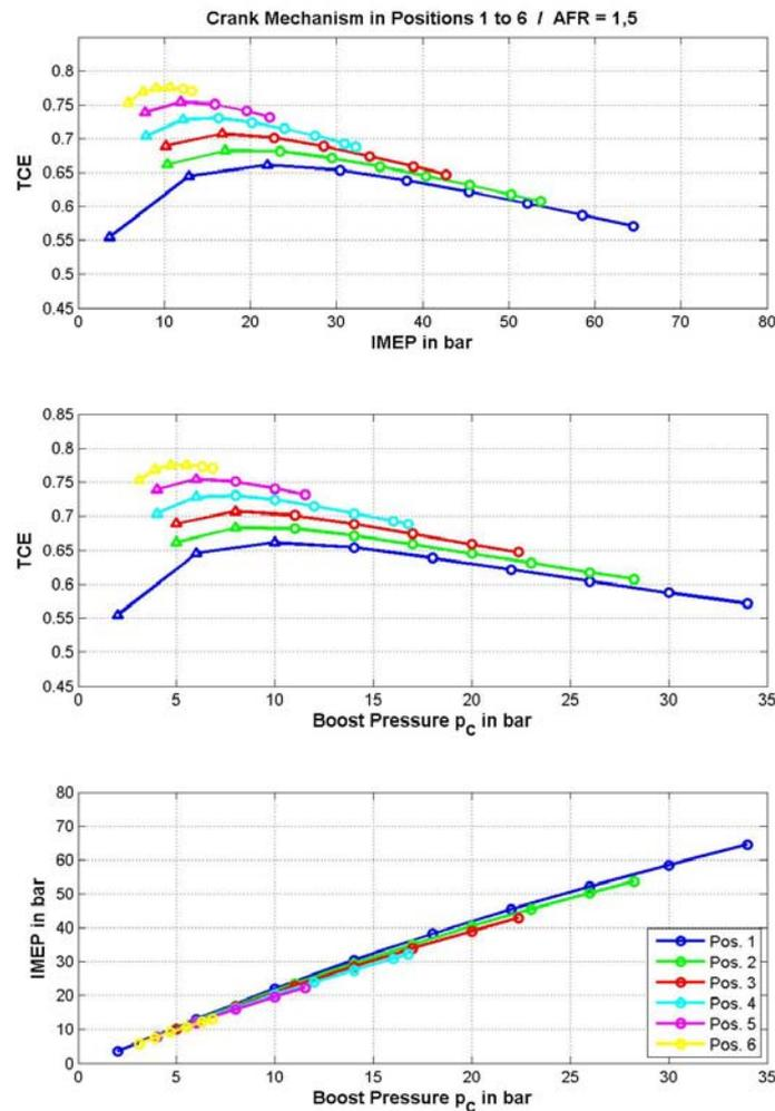
**Figure 16.** Correlation between TCE, IMEP, Boost Pressure and Crank Mechanism Positions at Full and many Part Loads with AFR = 1.5
