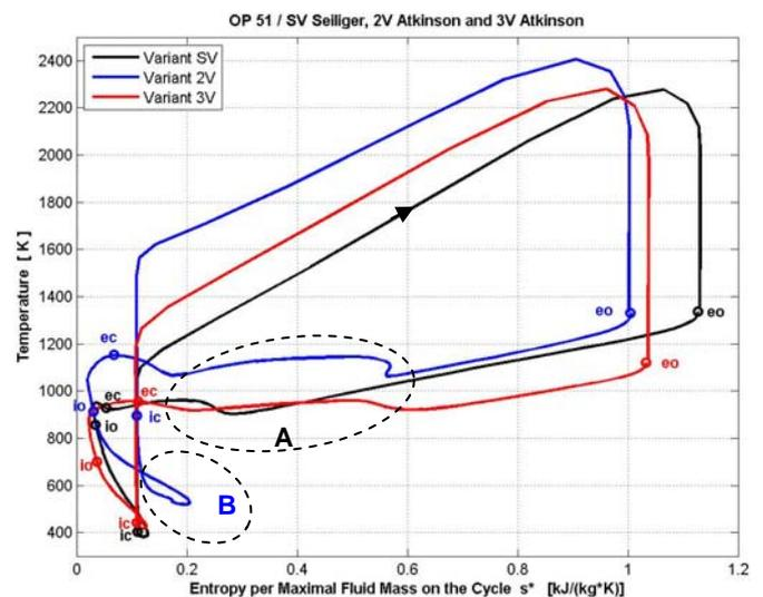
Figure 4. Temperature-specific\* Entropy (Entropy per Maximal Fluid Mass on the Cycle) Diagram (T, s\*)
