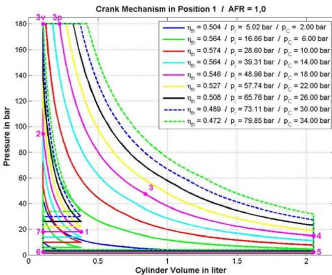
**Figure 13.** Pressure-Volume Diagrams for Crank Mechanism in Position 1, at many Loads, AFR = 1
